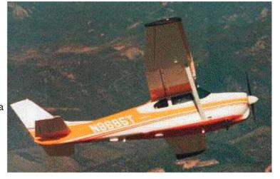
1960, the 210 was powered by a 260 horsepower fuel-injected six-cylinder engine that displaced 471 cubic inches. The 210 is the fastest single-engine airplane ever built by Cessna.
