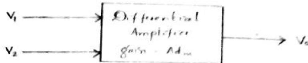
$$V_o = A_{dm} (V_1 - V_2)$$
