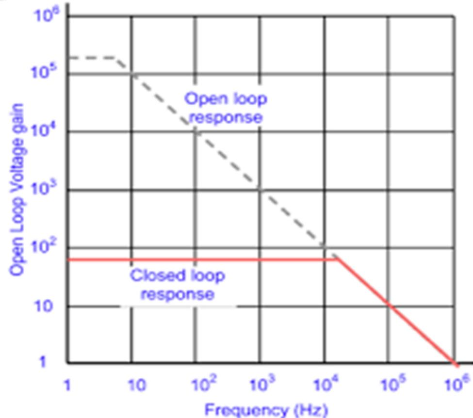
Product of the gain against frequency is constant at any point along the roll off curve for open loop and closed loop
