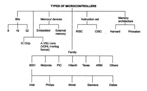
The microcontrollers are characterized regarding bus-width, instruction set, and memory structure. The types of microcontroller is shown in figure, they are characterized by their bits, memory architecture, memory/devices and instruction set
