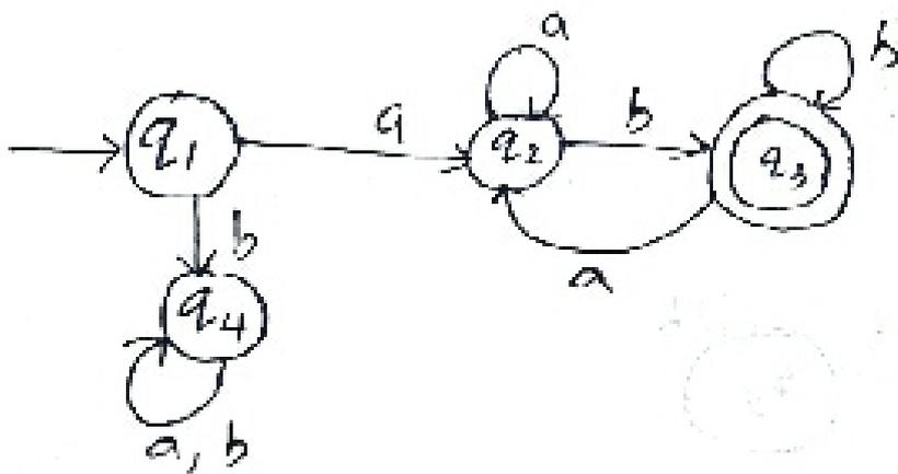
Q3) Construct a DFA which accepts set of all strings which starts and ends with different symbol when  $\Sigma = \{a,b\}$
